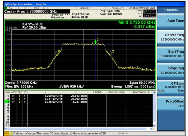
Test Mode:802.11ac VHT20 5720MHz Chain1 NII2C
