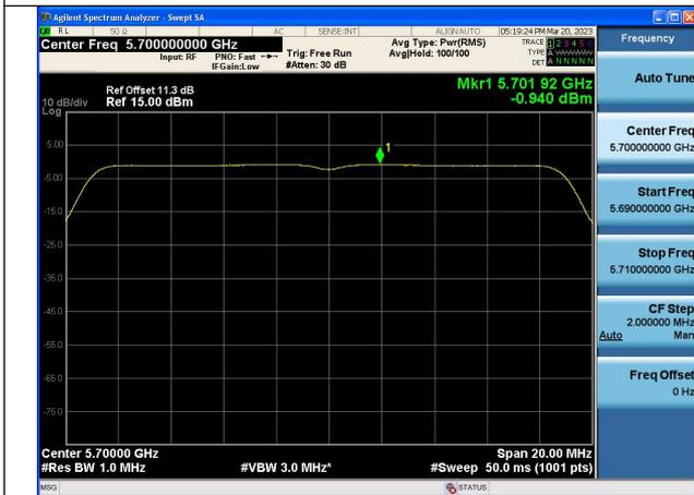
Mode:802.11ac VHT20 Frequency:5700MHz
