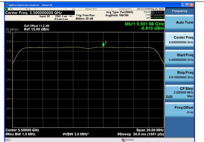
Mode:802.11ac VHT20 Frequency:5500MHz
