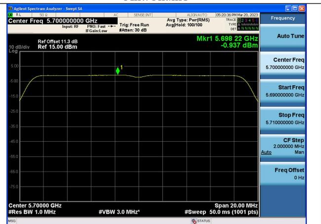
Mode:802.11ac VHT20 Frequency:5700MHz
