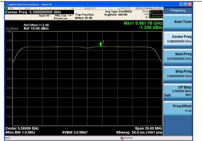
Mode:802.11ac VHT20 Frequency:5580MHz
