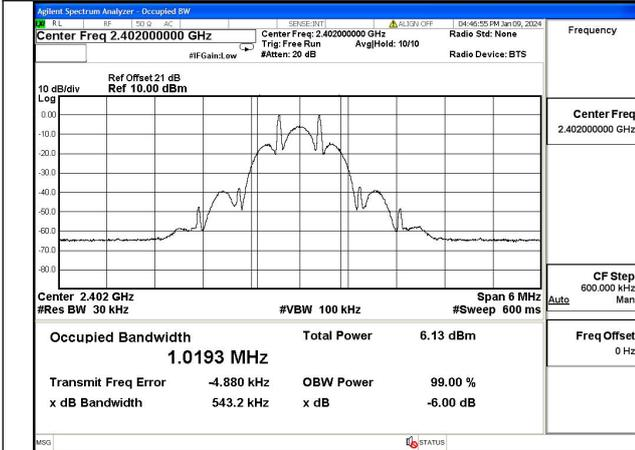
Test Mode:Coded 125K 2402MHz
