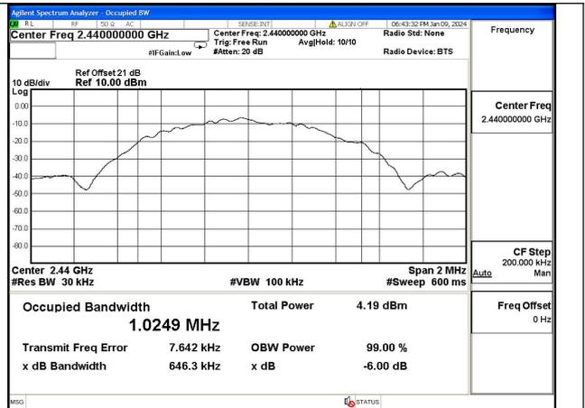
Test Mode:GFSK (LE 1Mbps) 2402MHz
