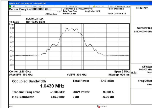
Test Mode:Coded 125K 2480MHz
