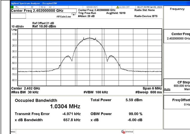
Test Mode:Coded 500K 2402MHz
