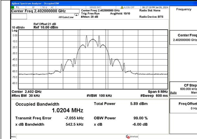
Test Mode:Coded 125K 2402MHz
