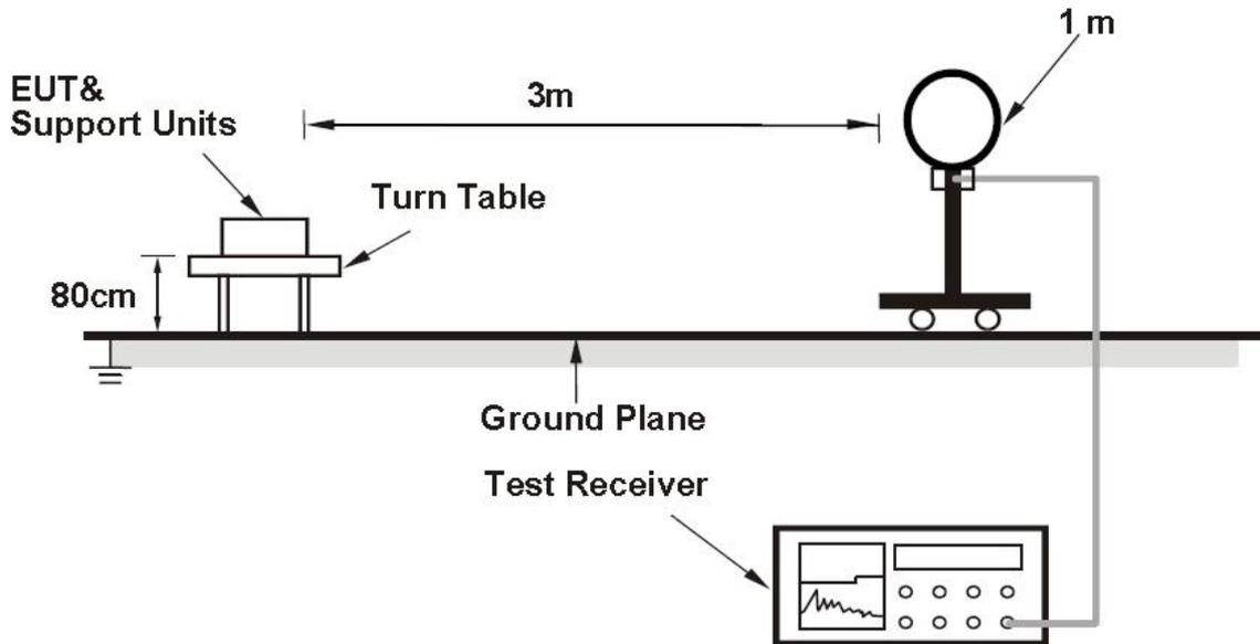
For Radiated emission 30MHz to 1GHz
