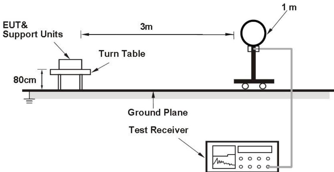
**For Radiated emission 30MHz to 1GHz**
