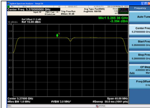
Mode:802.11ac VHT40 Frequency:5270MHz
