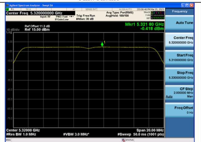
Mode:802.11ac VHT20 Frequency:5320MHz
