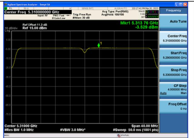
Mode:802.11ac VHT40 Frequency:5310MHz
