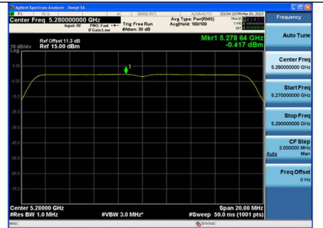
Mode:802.11ac VHT20 Frequency:5280MHz
