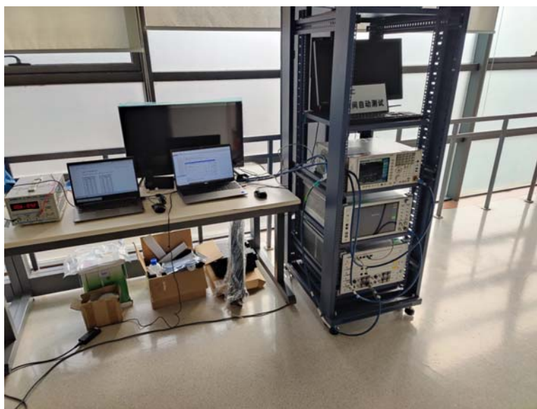
RF Conducted Test setup (LTE/NR)
