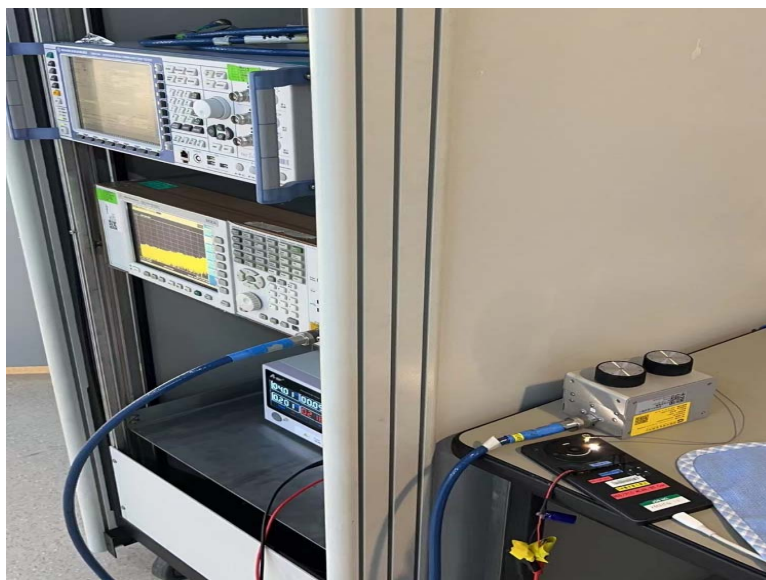
RF Conducted Test setup (BT/WIFI)
