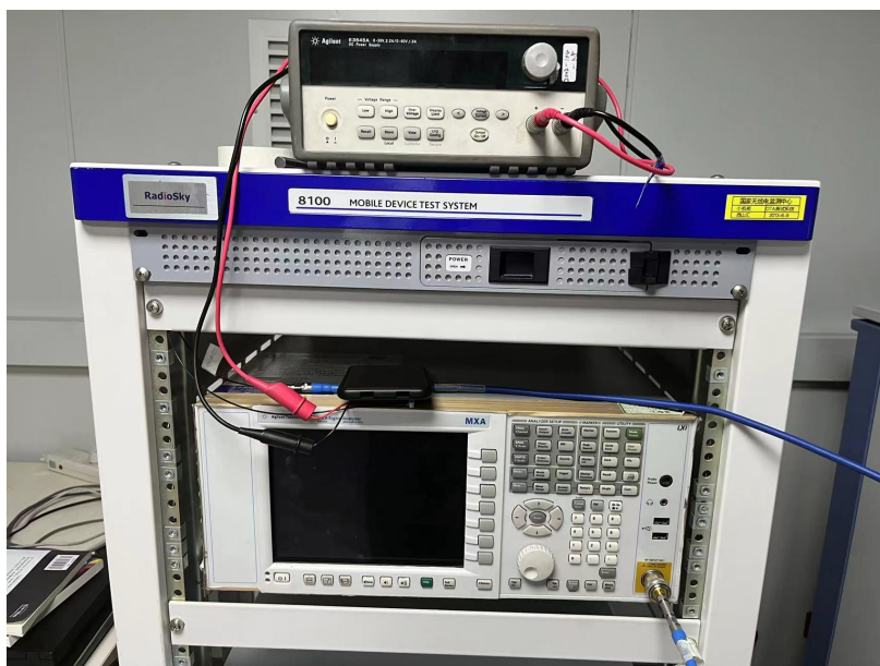
RF Conducted Test setup (BLE)
