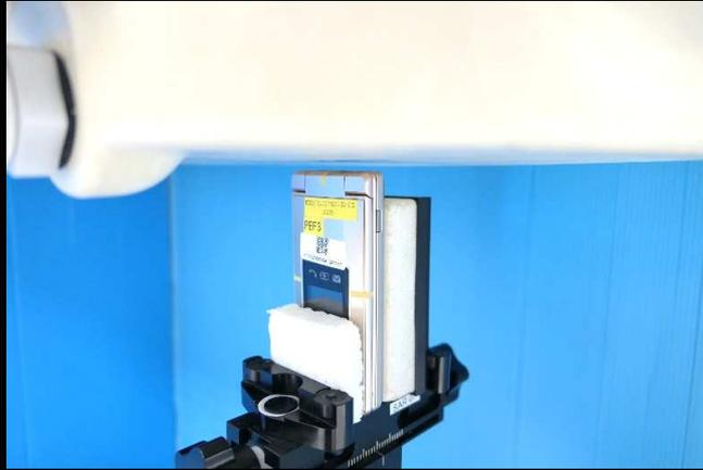
**Top Side of EUT Tested at 10 mm**
