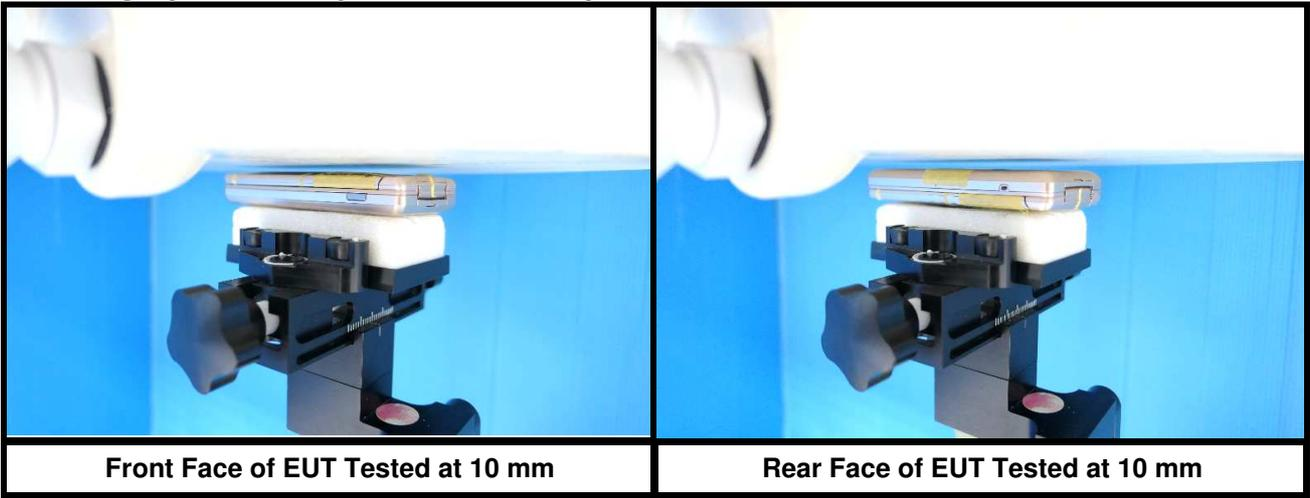
**<Photographs of Hospot SAR Test Setup>**
