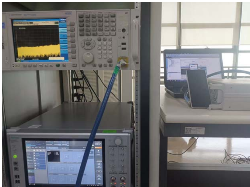
RF Conducted Test setup (GSM/WCDMA/LTE)
