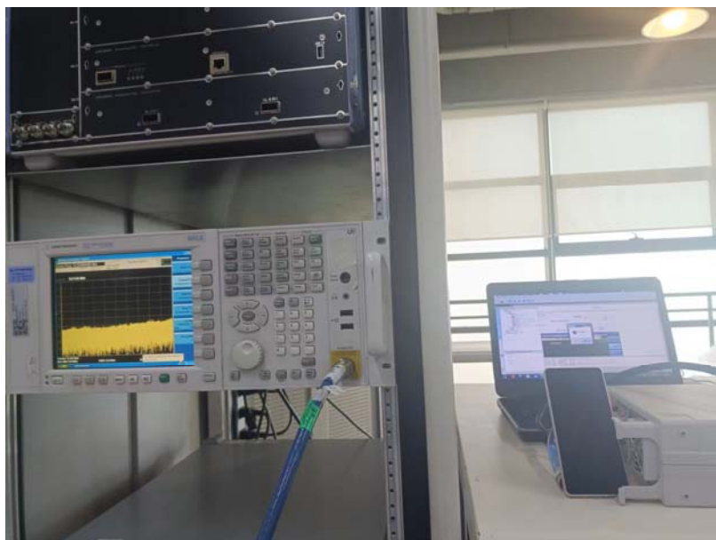
RF Conducted Test setup (BT/WIFI)
