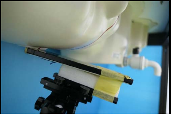
Right Tilted of EUT Tested at 0 mm
