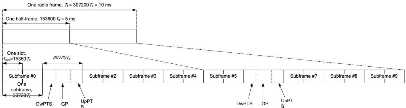
3GPP TS 36.211 Figure 4.2-1: Frame Structure Type 2
