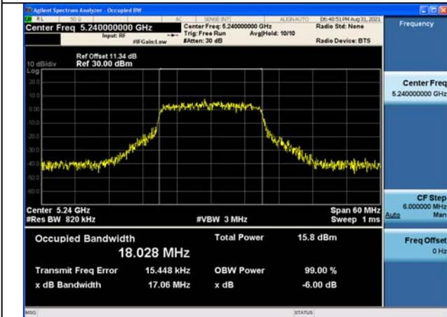
Test Mode:802. 11ac VHT40
