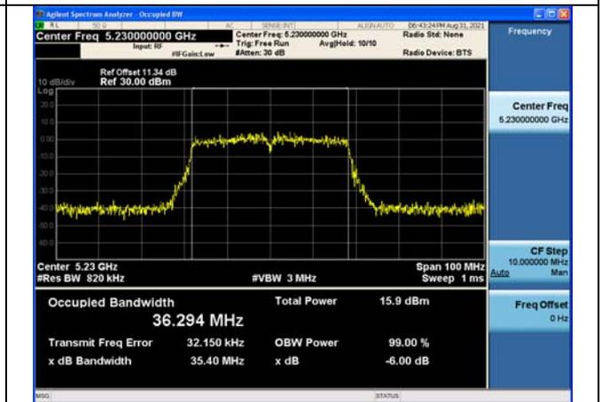
Test Mode:802. 11ac VHT20
