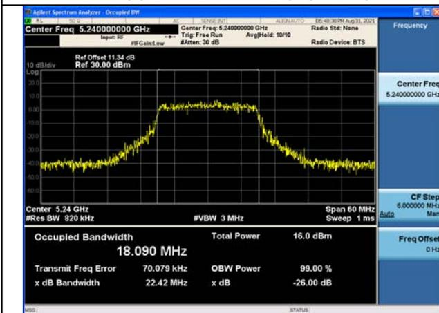
Test Mode:802. 11ac VHT40
