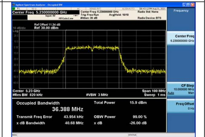
Test Mode:802. 11ac VHT20
