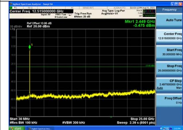
Test Mode:802. 11n HT40 Chain0 CH9
