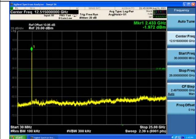
Test Mode:802. 11n HT20 Chain0 CH11
