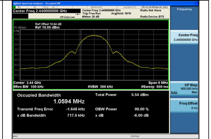
Test Mode:Coded 125K MHz
