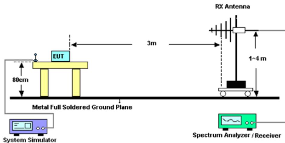
For radiated test above 1GHz
