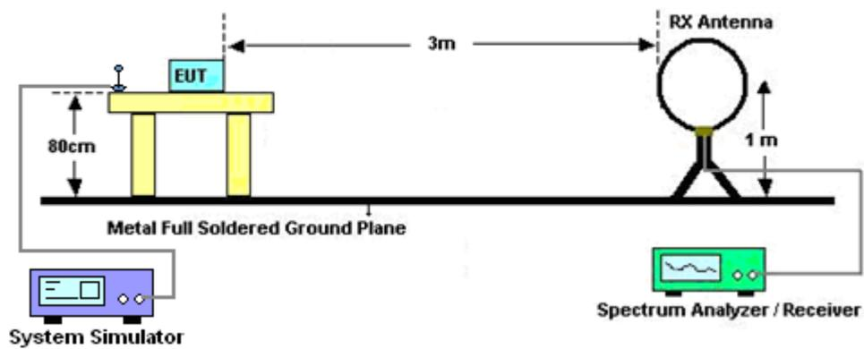
For radiated test from 30MHz to 1GHz
