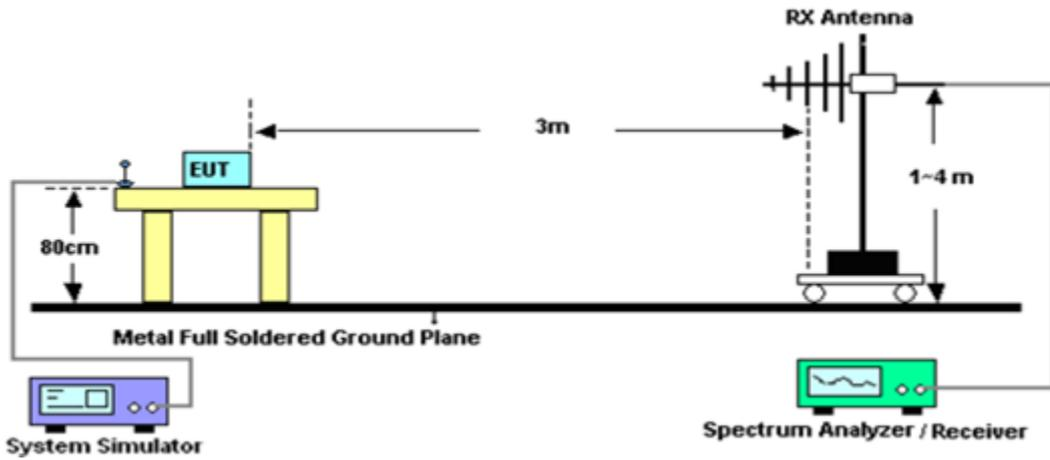
For radiated test above 1GHz
