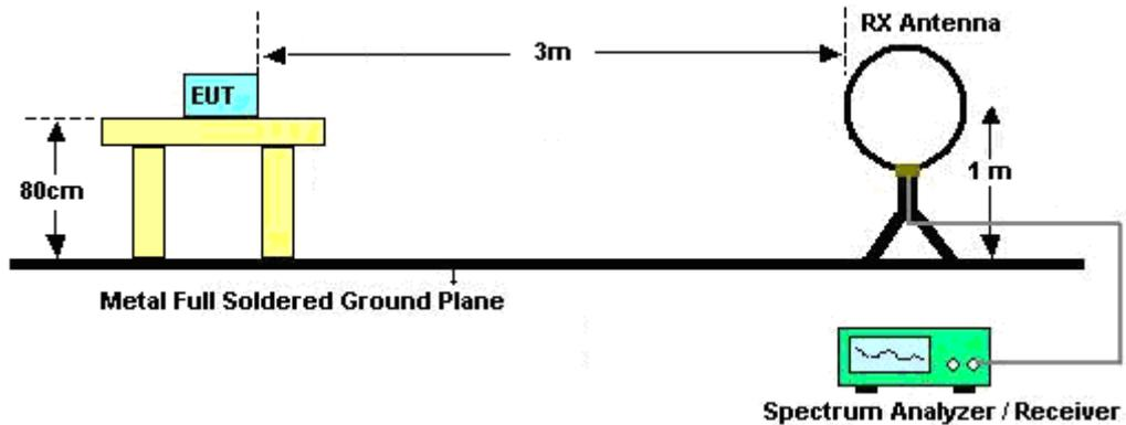
For radiated emissions from 30MHz to 1GHz
