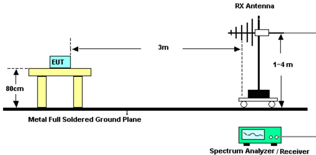
For radiated test above 1GHz
