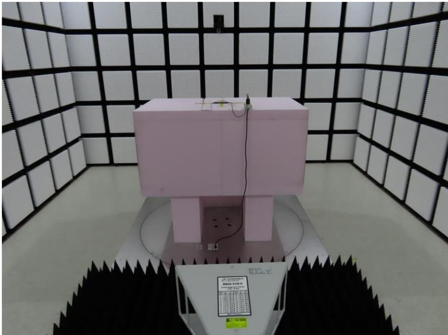
Z Plane for Bluetooth – LE 2Mbps + WLAN 802.11ac VHT80 +
