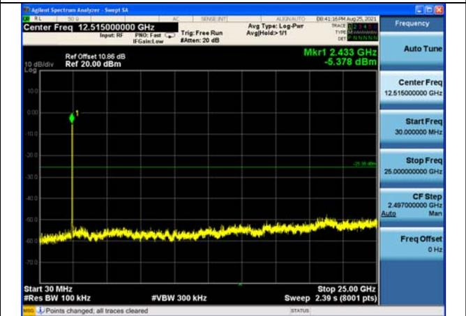
Test Mode:802. 11n HT40 Chain0 CH9
