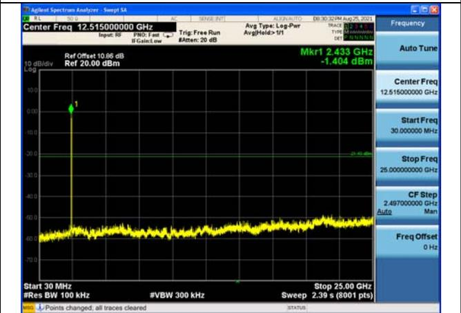
Test Mode:802. 11n HT20 Chain0 CH11
