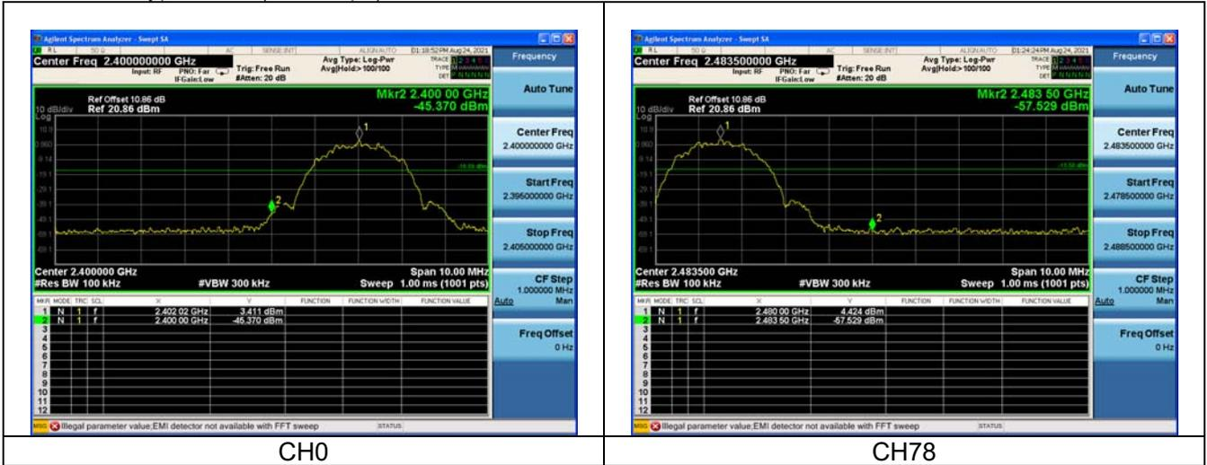
Offset 1.2dB = Temporary antenna connector loss 0.2dB+ Cable loss 1.0dB
