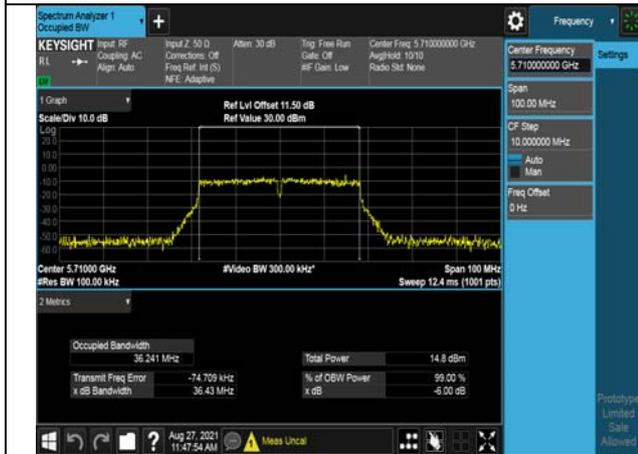
Test Mode:802. 11ac VHT80
