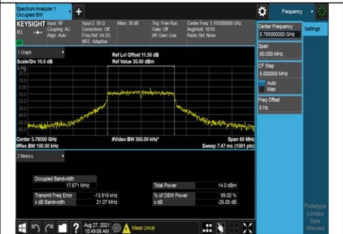
Test Mode:802. 11ac VHT20 Chain0
