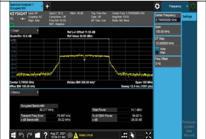
Test Mode:802. 11ac VHT40 Chain0
