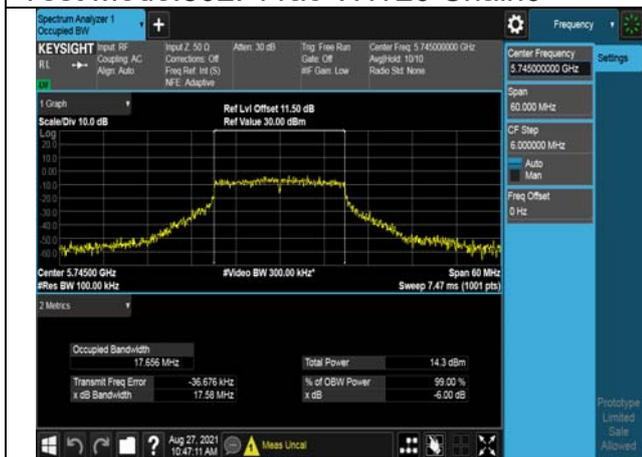
Test Mode:802. 11ac VHT20 Span Chain0
