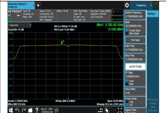
Test Mode:802. 11ac VHT20 Chain0
