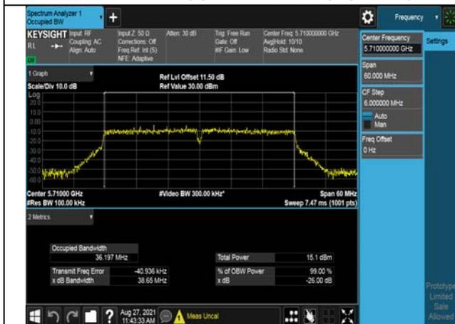
Test Mode:802. 11ac VHT20
