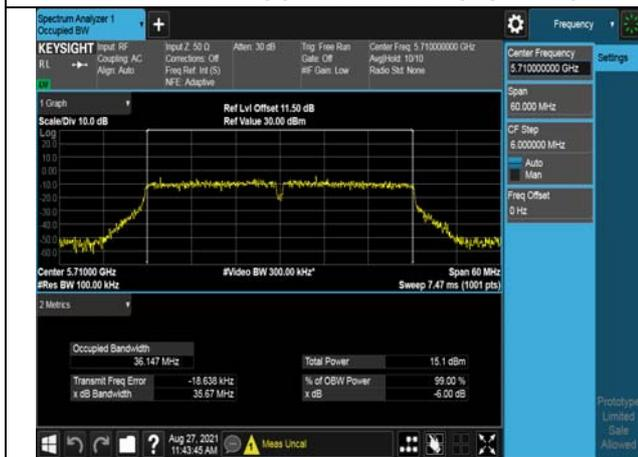
Test Mode:802. 11ac VHT20
