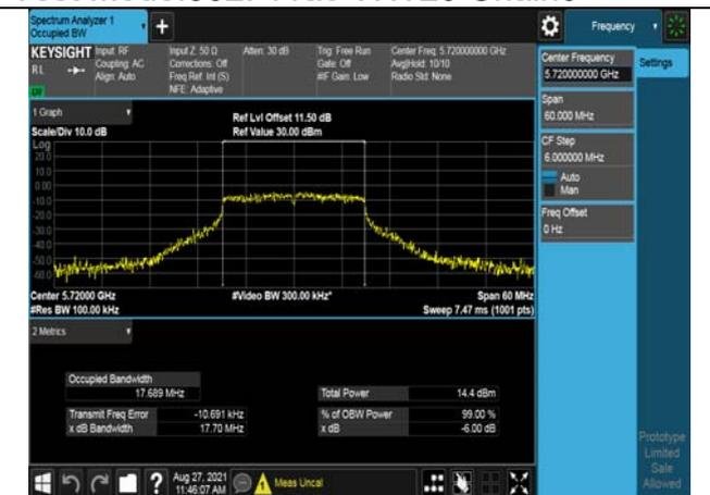
Test Mode:802. 11ac VHT40
