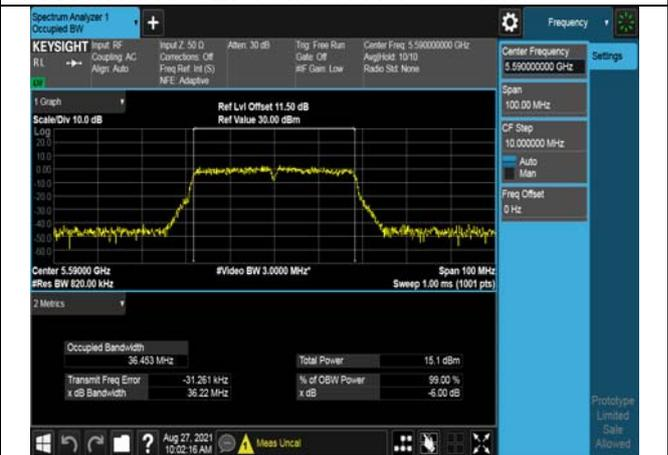
Test Mode:802. 11ac VHT40 Chain0
