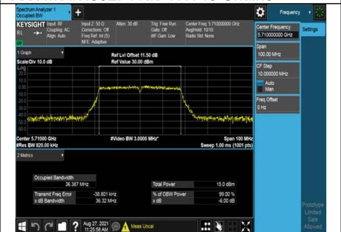
Test Mode:802. 11ac VHT80
