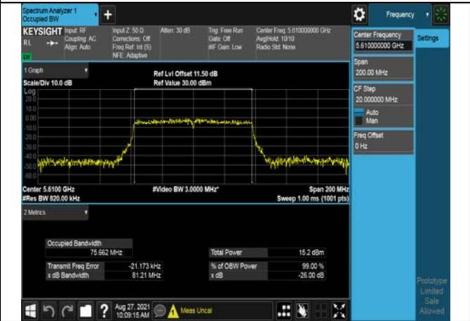
Test Mode:802. 11ac VHT80 Chain0
