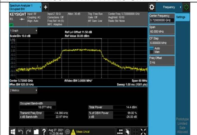
Test Mode:802. 11ac VHT40
