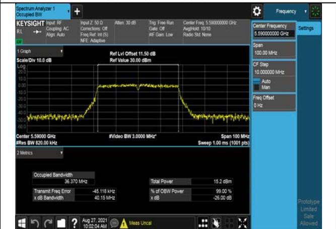
Test Mode:802. 11ac VHT40 Chain0
