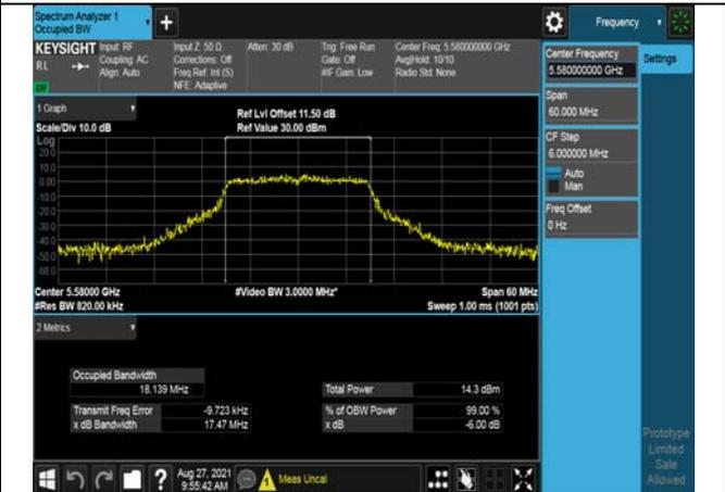
Test Mode:802. 11ac VHT20 Chain0
