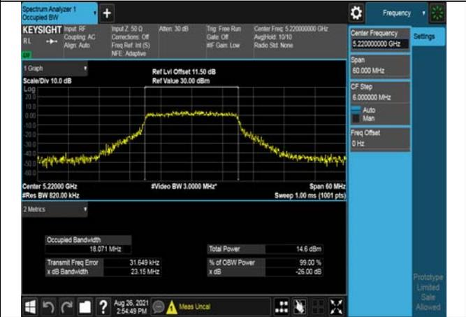
Test Mode:802. 11ac VHT20 Chain0
