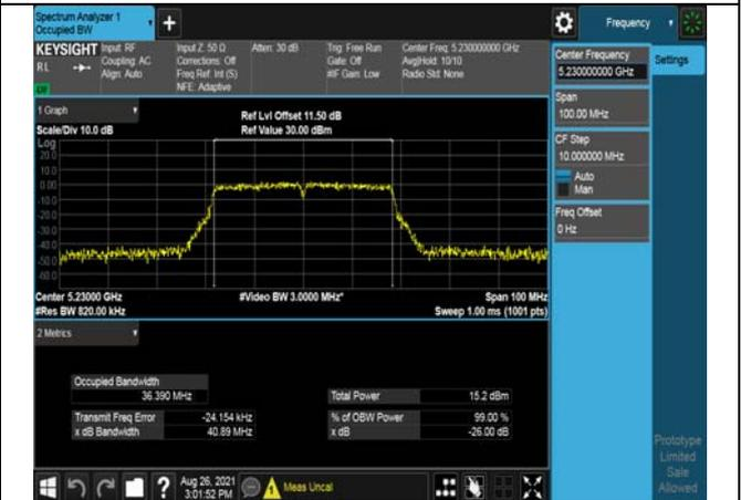
Test Mode:802. 11ac VHT80
