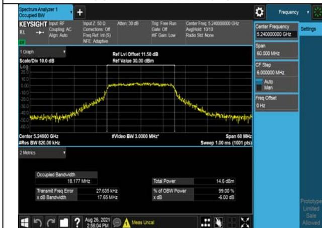
Test Mode:802. 11ac VHT40
