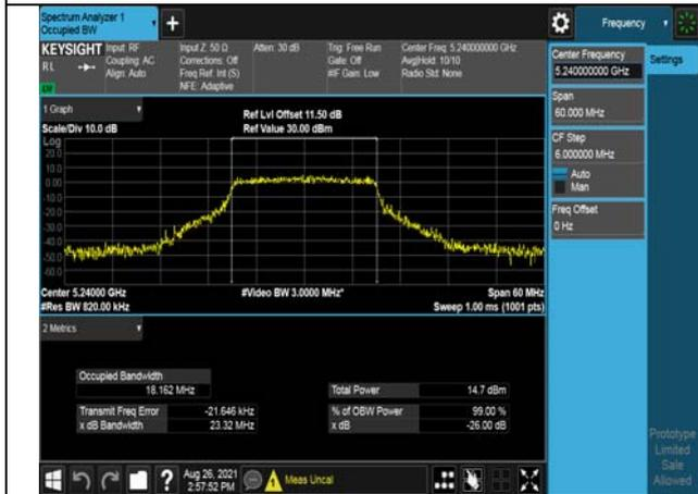
Test Mode:802. 11ac VHT40
