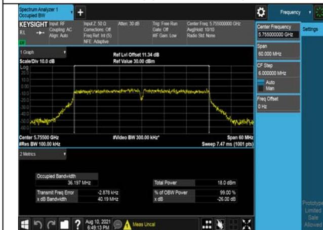
Test Mode:802. 11ac VHT20
