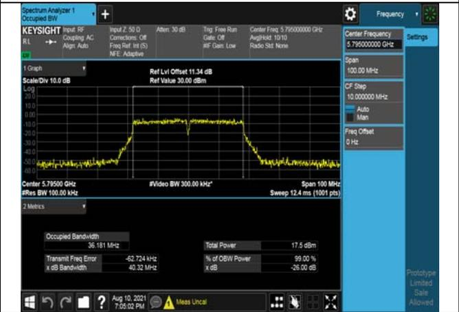
Test Mode:802. 11ac VHT40 Ant7
