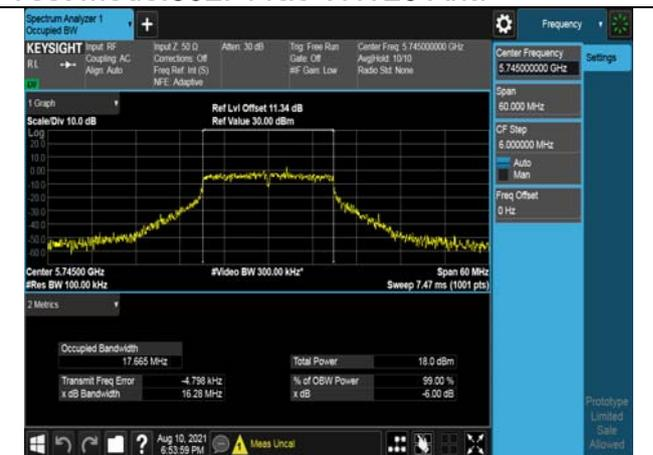
Test Mode:802. 11ac VHT40
