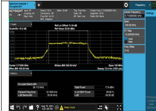
Test Mode:802. 11ac VHT40 Ant7
