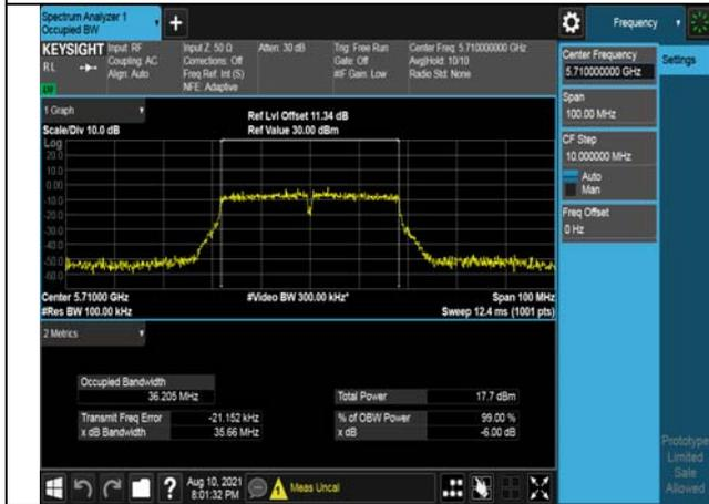
Test Mode:802. 11ac VHT40 Ant7
