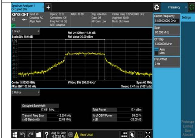
Test Mode:802. 11ac VHT20 Ant7
