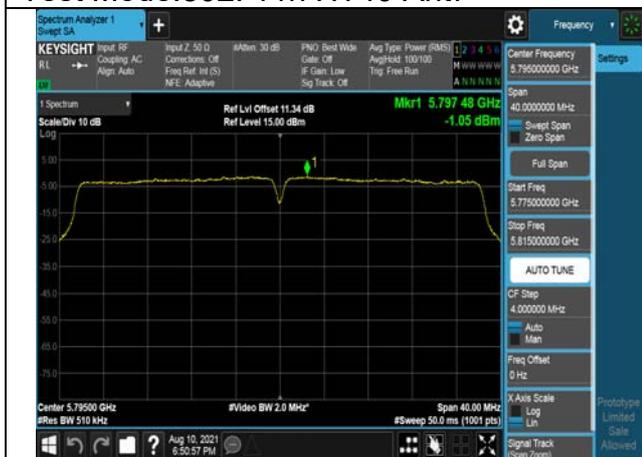
Test Mode:802. 11ac VHT20
