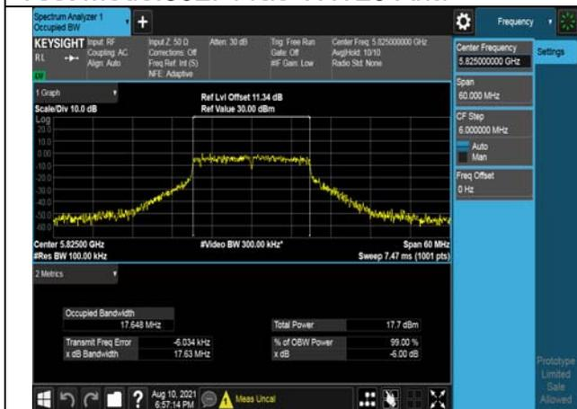
Test Mode:802. 11ac VHT20 Ant7
