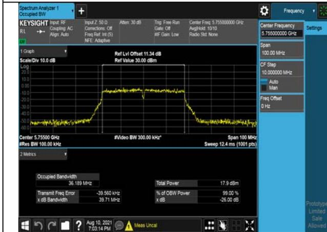
Test Mode:802. 11ac VHT80
