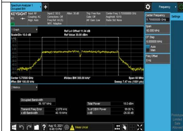
Test Mode:802. 11ac VHT20
