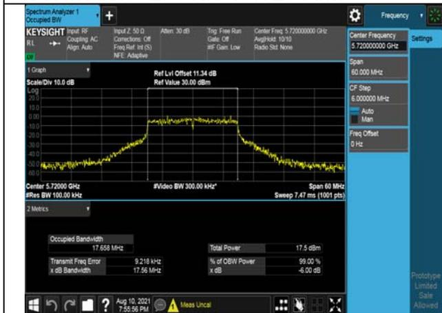
Test Mode:802. 11ac VHT20 Ant7
