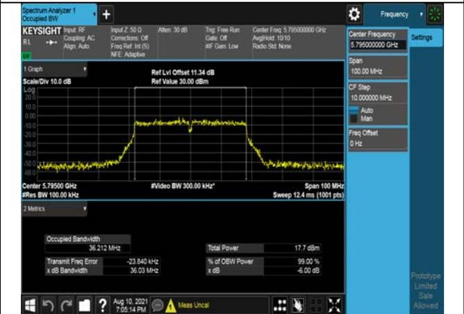
Test Mode:802. 11ac VHT40 Ant7
