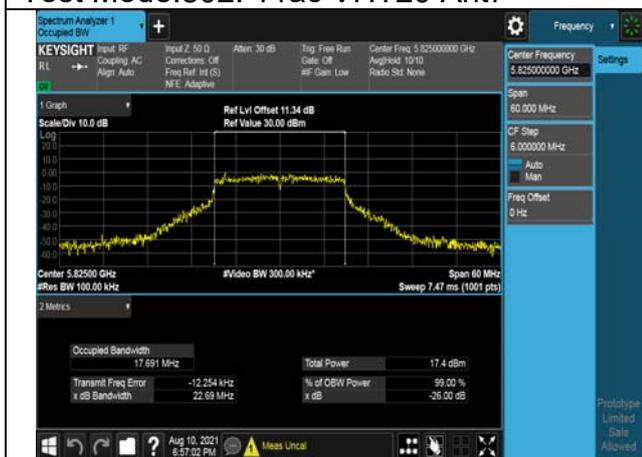
Test Mode:802. 11ac VHT20 Ant7
