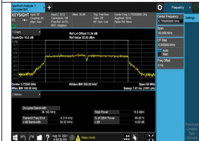
Test Mode:802. 11ac VHT20
