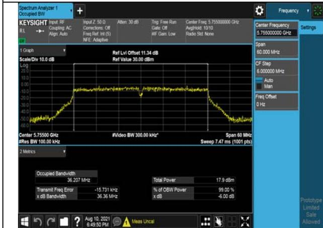
Test Mode:802. 11ac VHT20
