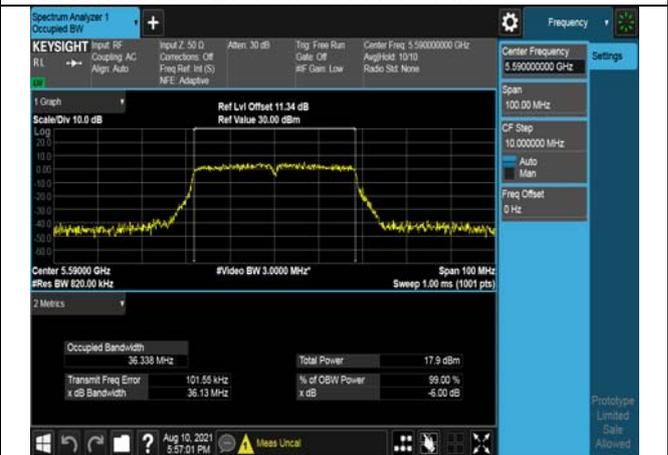
Test Mode:802. 11ac VHT40 Ant7
