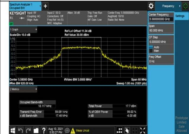
Test Mode:802. 11ac VHT20 Ant7
