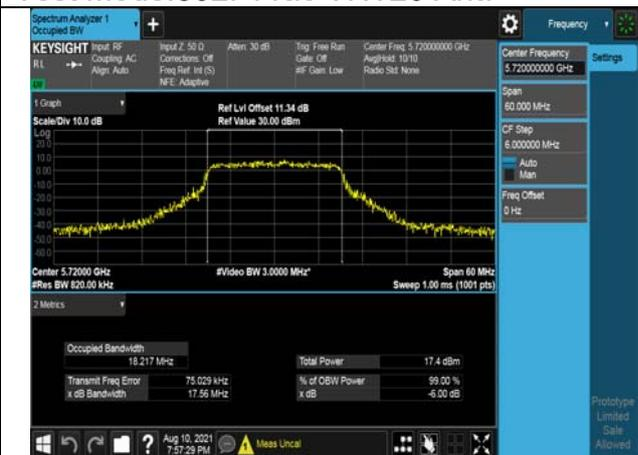
Test Mode:802. 11ac VHT40
