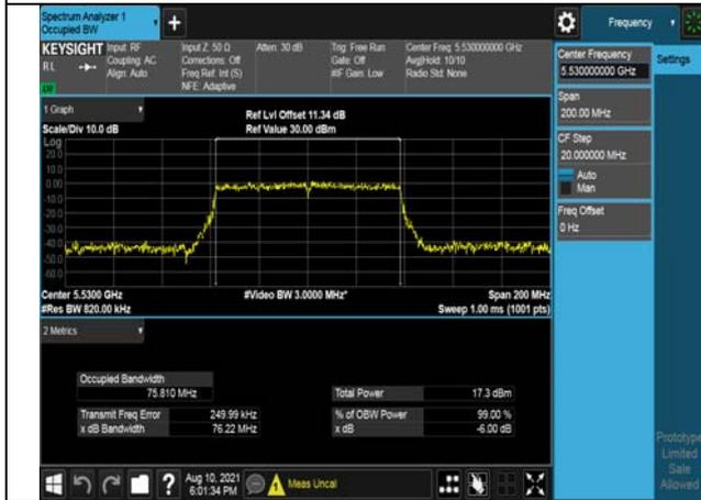
Test Mode:802. 11ac VHT80 Ant7
