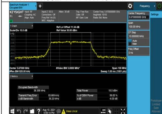
Test Mode:802. 11ac VHT40 Ant7
