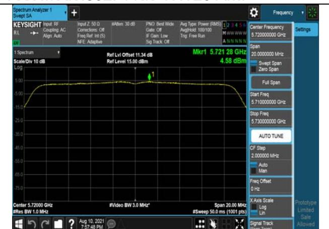
Test Mode:802. 11ac VHT40
