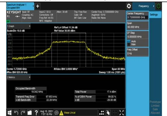
Test Mode:802. 11ac VHT40
