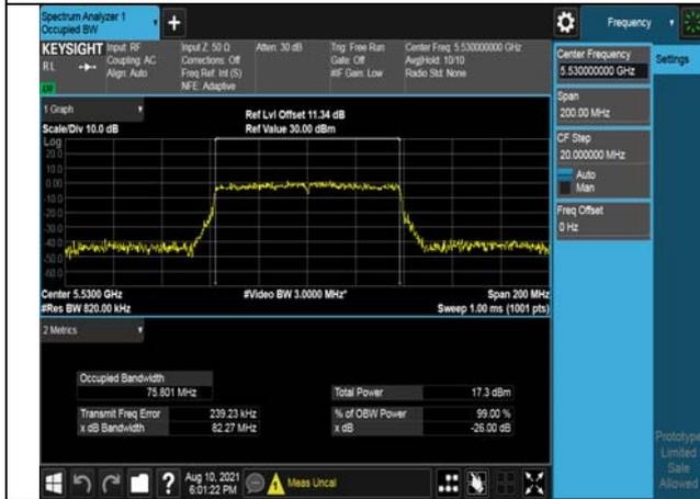
Test Mode:802. 11ac VHT80 Ant7
