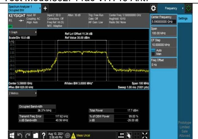
Test Mode:802. 11ac VHT40 Ant7
