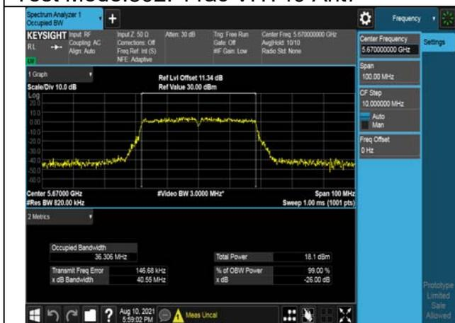
Test Mode:802. 11ac VHT40 Ant7
