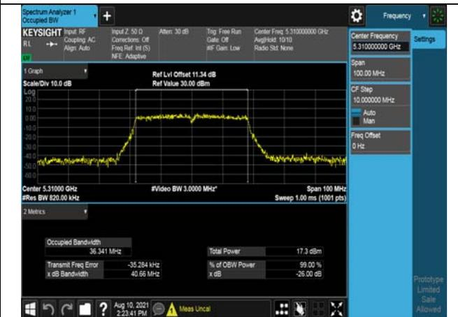
Test Mode:802. 11ac VHT20
