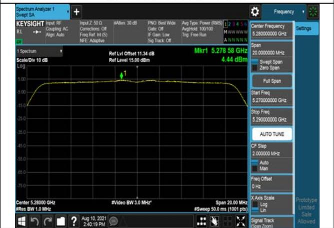
Test Mode:802. 11ac VHT20 Ant7
