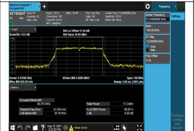
Test Mode:802. 11ac VHT20
