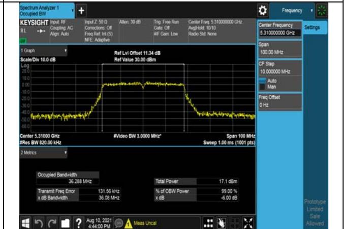
Test Mode:802. 11ac VHT80
