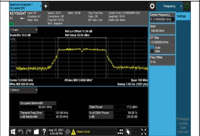
Test Mode:802. 11ac VHT80
