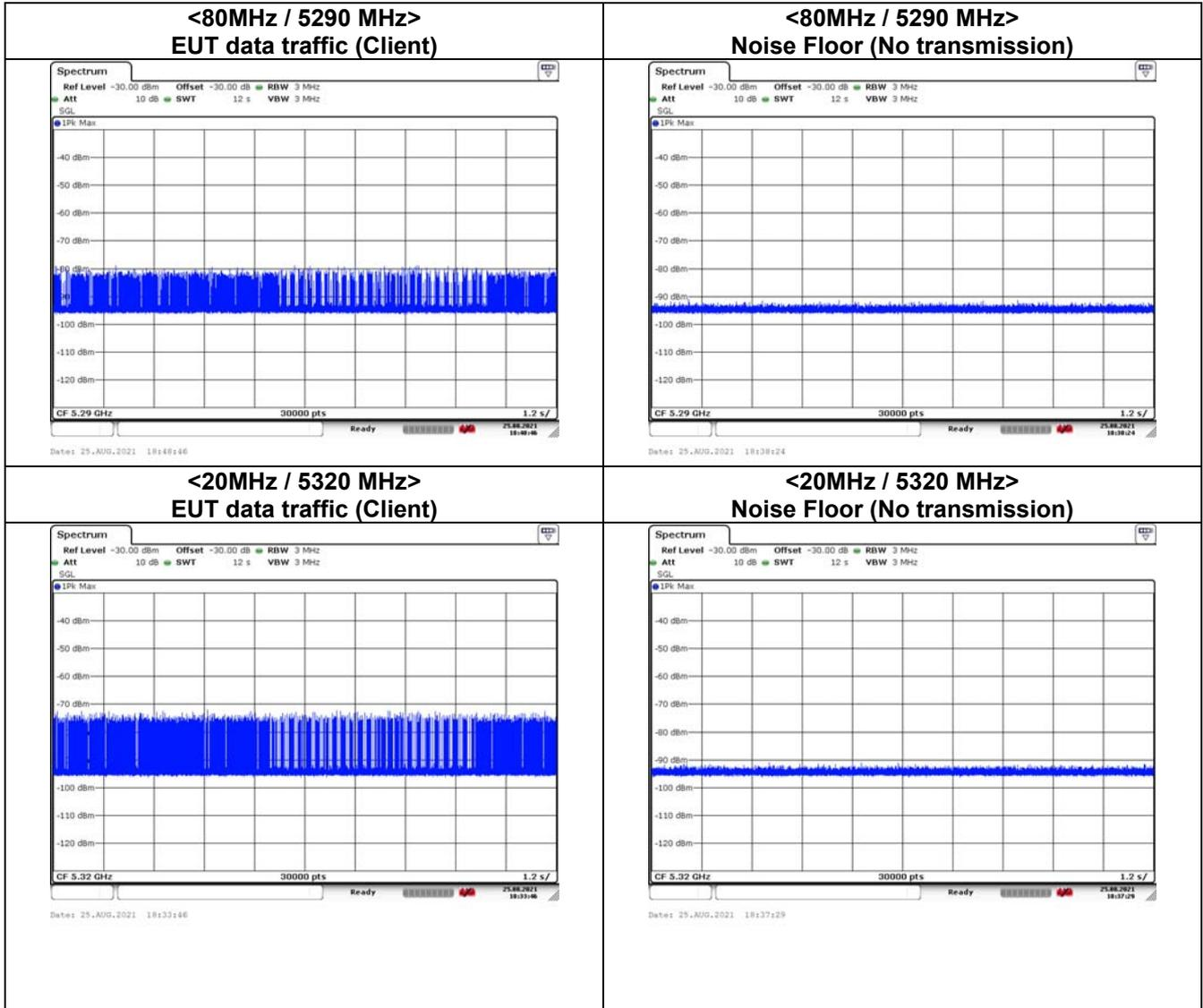
**Channel Move Time, Channel Closing Transmission Time and Non-Occupancy Period for Client Beacon Test**
