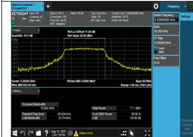
Test Mode:802. 11ac VHT40
