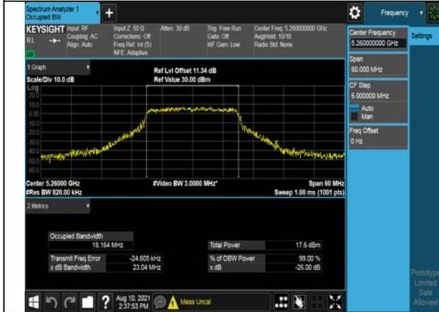
Test Mode:802. 11ac VHT20 Ant7
