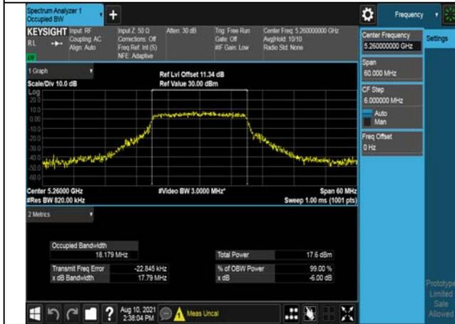
Test Mode:802. 11ac VHT20 Ant7
