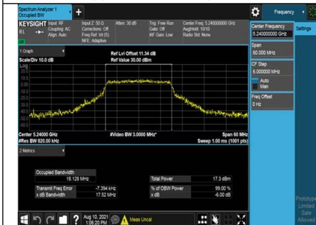
Test Mode:802. 11ac VHT40
