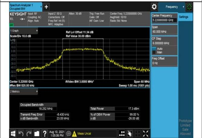
Test Mode:802. 11ac VHT20 Ant7
