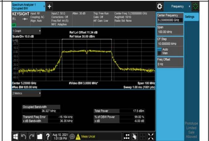
Test Mode:802. 11ac VHT20
