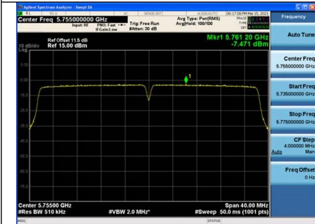
Test Mode:802. 11ac VHT40 Ant7
