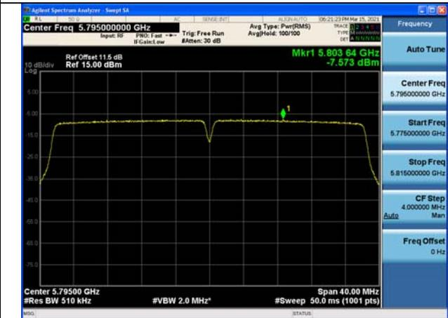
Test Mode:802. 11ac VHT40 Ant8
