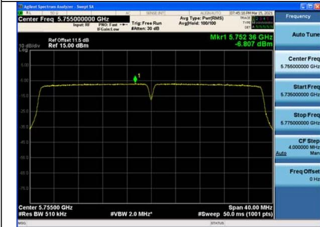
Test Mode:802. 11ac VHT40 Ant8
