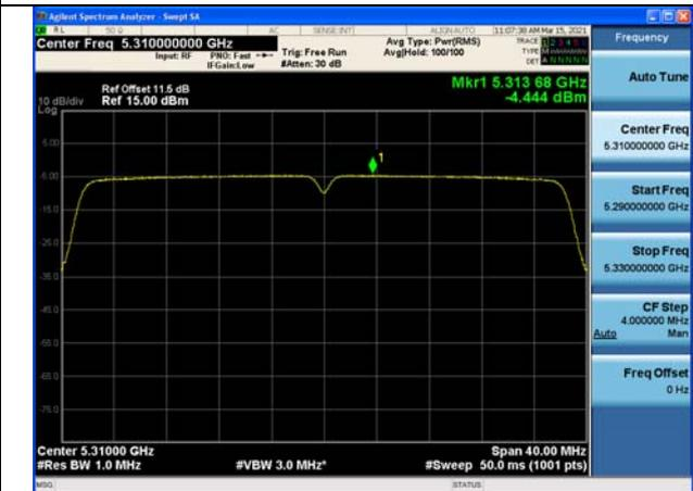
Test Mode:802. 11ac VHT20
