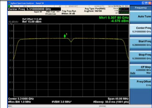
Test Mode:802. 11ac VHT80
