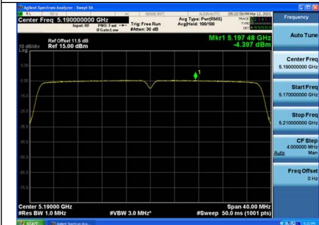
Test Mode:802. 11ac VHT40 Ant8
