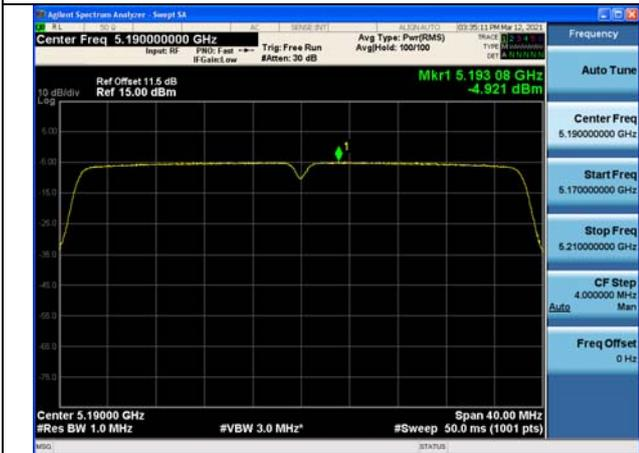
Test Mode:802. 11ac VHT40 Ant7
