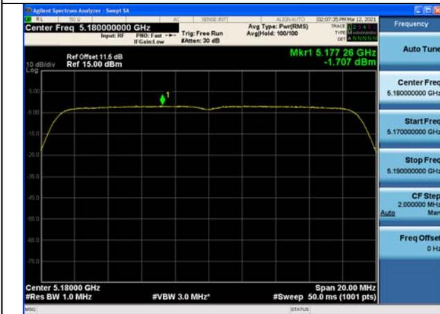
Test Mode:802. 11ac VHT20 Ant7
