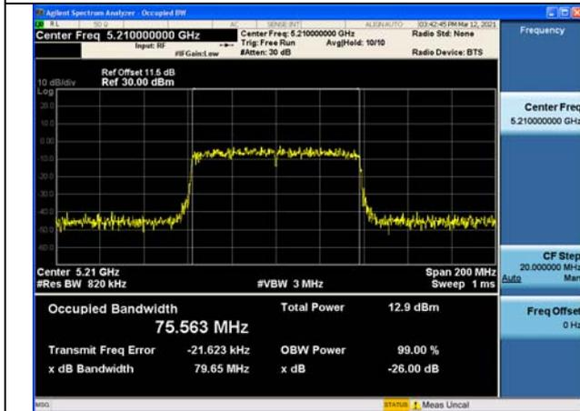
Test Mode:802. 11ac VHT80 Ant8
