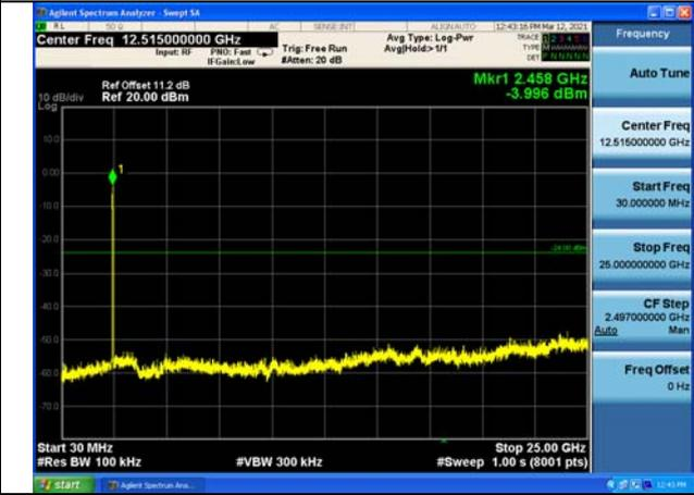
**Band edge measurement (RF Conducted measurement)**
