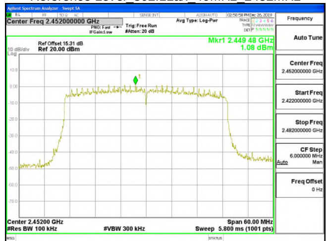
Reference Level 802.11ax 40MHz 2452MHz
