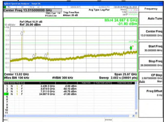
Spurious Emission 802.11ax 20MHz 2462MHz
