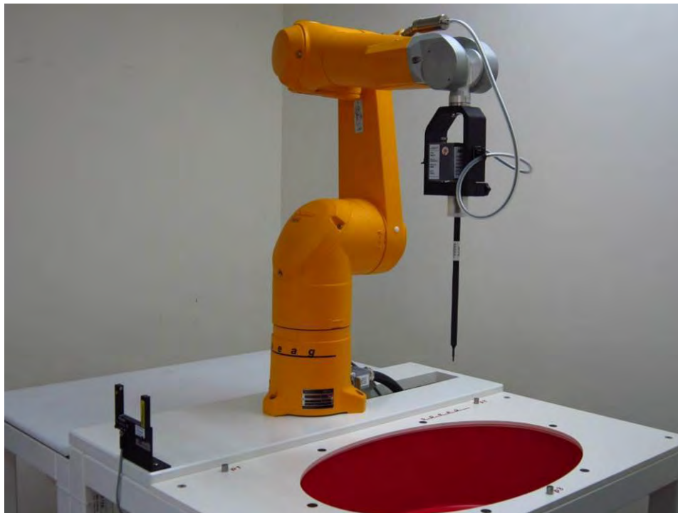
Fig.1 Photograph of the SAR measurement system
