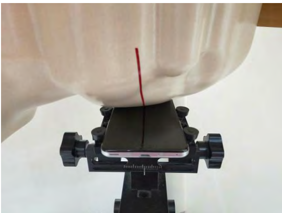
Fig.5 Left Head Section / Cheek-Touch Position
