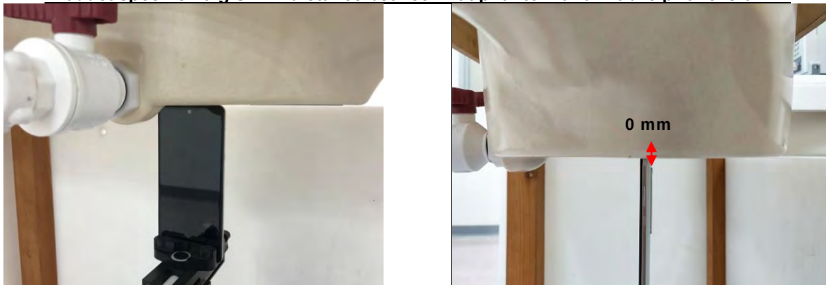
Fig.18 EUT Top side to flat phantom
