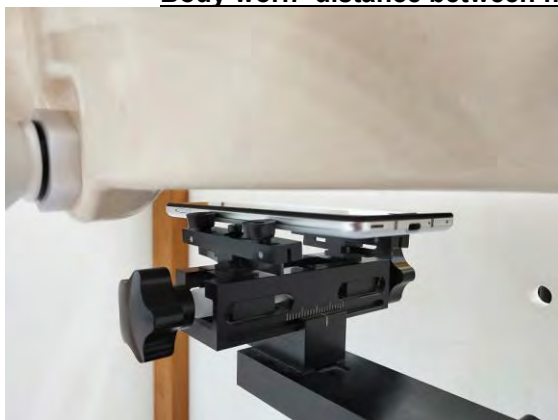
Fig.7 EUT Front side to flat phantom
