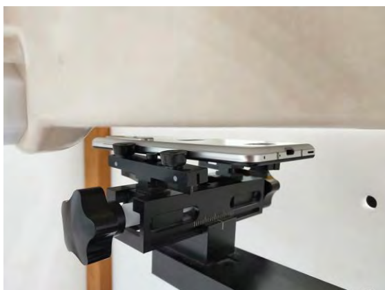
Fig.8 EUT Back side to flat phantom
