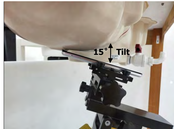
Fig.4 Right Head Section / Ear-Tilt Position(15°)
