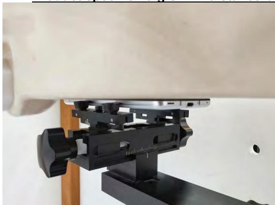
Fig.15 EUT Front side to flat phantom
