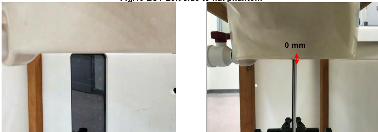
Fig.20 EUT Bottom side to flat phantom
