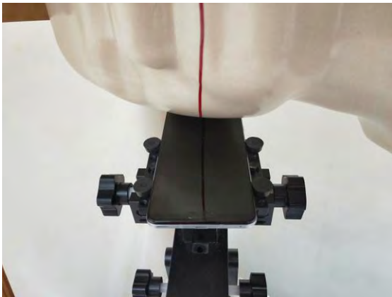
Fig.4 Right Head Section / Ear-Tilt Position(15°)
