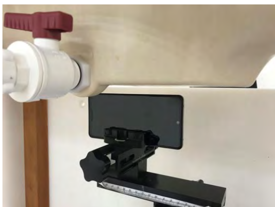
Fig.13 EUT Left side to flat phantom
