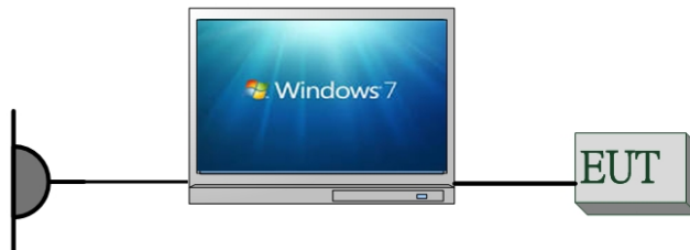
Fig. 2-1 Radiated Emission Configuration (NFC & BT & BLE & WLAN)
