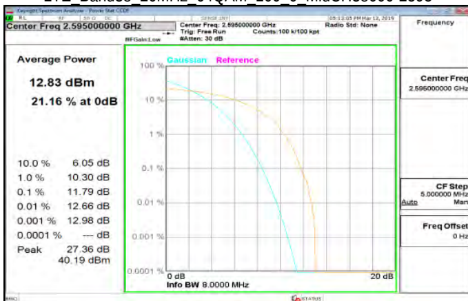
LTE Band38 20MHz 64QAM 100 0 MidCH38000-2595
