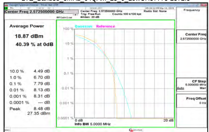
LTE Band38 5MHz 64QAM 25 0 MidCH38000-2595
