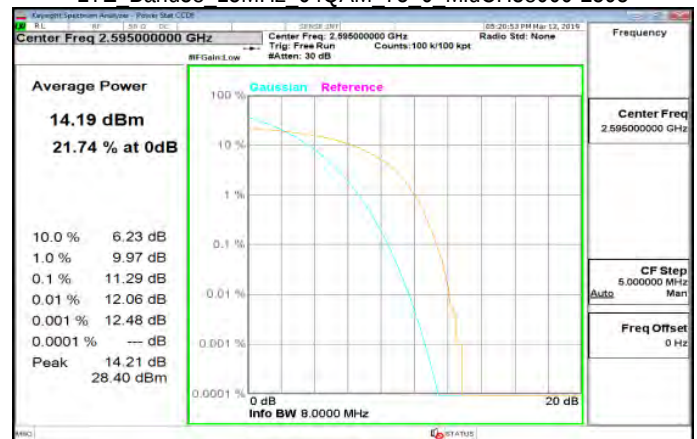
LTE Band38 15MHz 64QAM 75 0 MidCH38000-2595
