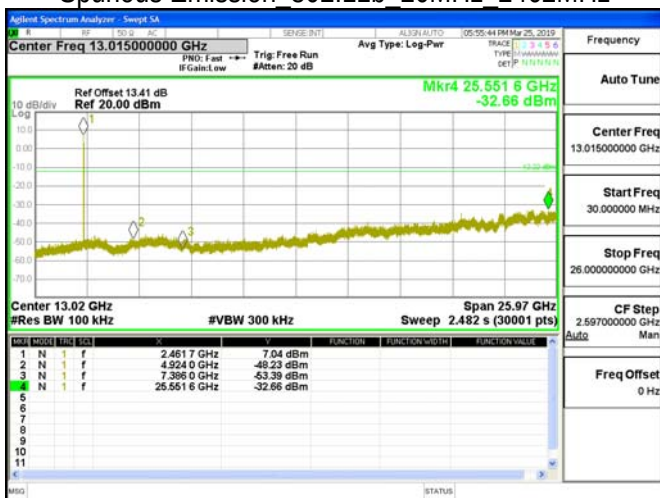
Spurious Emission 802.11b 20MHz 2462MHz
