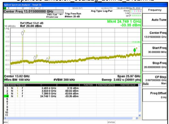
Spurious Emission 802.11g 20MHz 2462MHz
