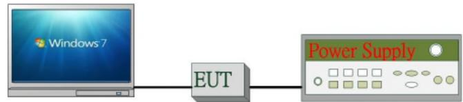
Fig. 2-2 AC Power Line Conducted Emission
