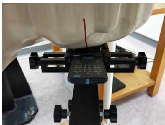
Fig.5 Left Head Section / Cheek-Touch Position
