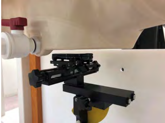
Fig.7 EUT Front side to flat phantom
