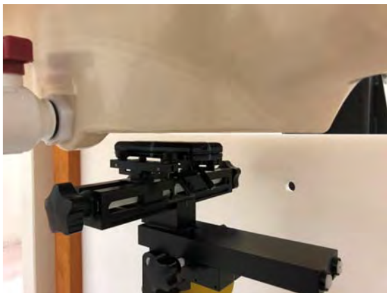
Fig.10 EUT Back side to flat phantom
