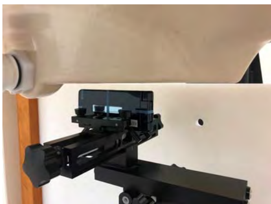
Fig.13 EUT Left side to flat phantom
