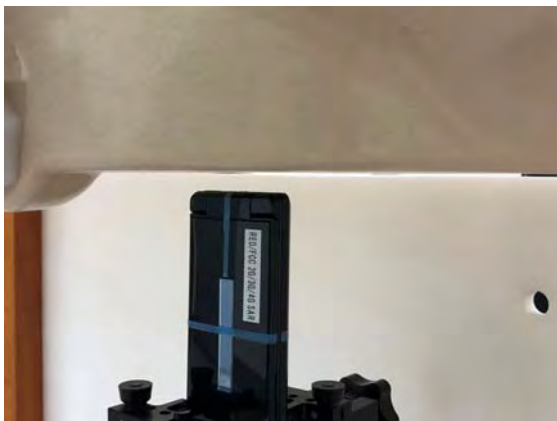
Fig.11 EUT Top side to flat phantom
