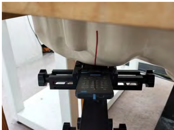
Fig.3 Right Head Section / Cheek-Touch Position
