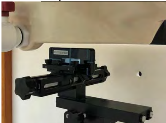
Fig.12 EUT Right side to flat phantom
