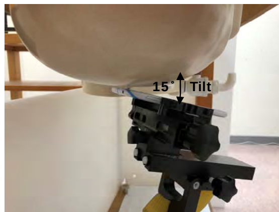
Fig.4 Right Head Section / Ear-Tilt Position(15°)
