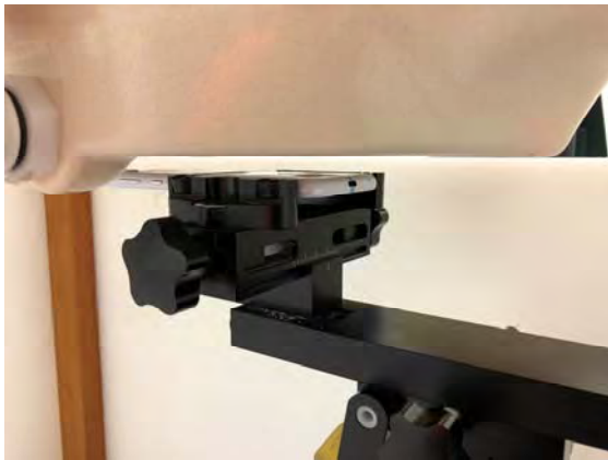
Fig.8 EUT Back side to flat phantom
