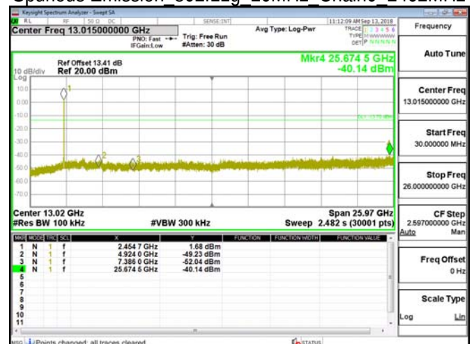
Spurious Emission 802.11g 20MHz Chain0 2462MHz
