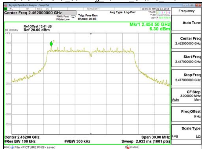
Reference Level 802.11g 20MHz Chain0 2462MHz
