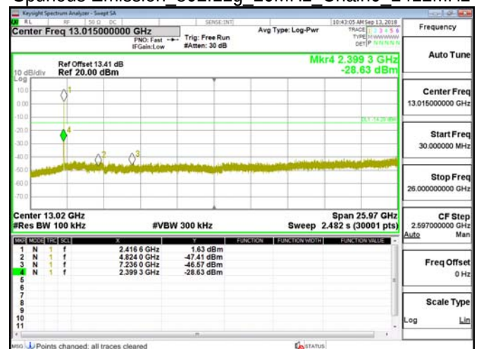
Spurious Emission 802.11g 20MHz Chain0 2437MHz
