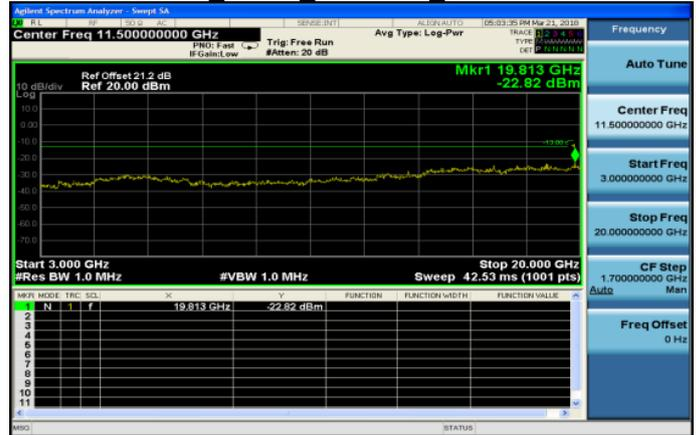
3GHz~10GHz GPRS 1900MHz LowCH512-1850.2
