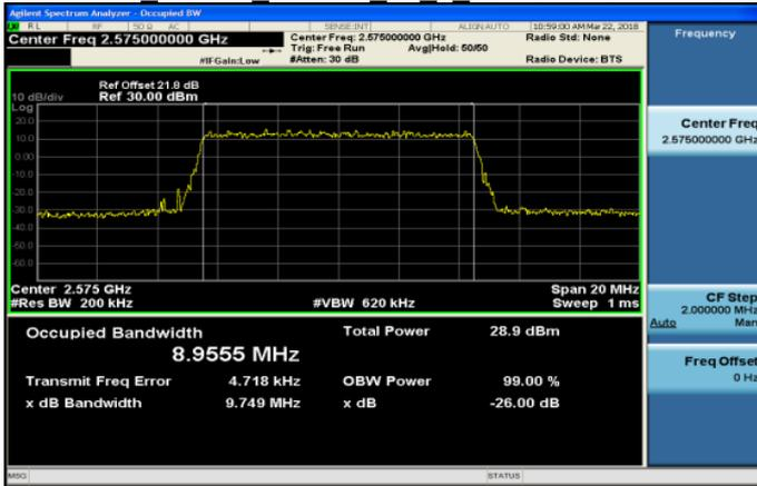
Band38 10MHz 64QAM 50 0 LowCH37800-2575
