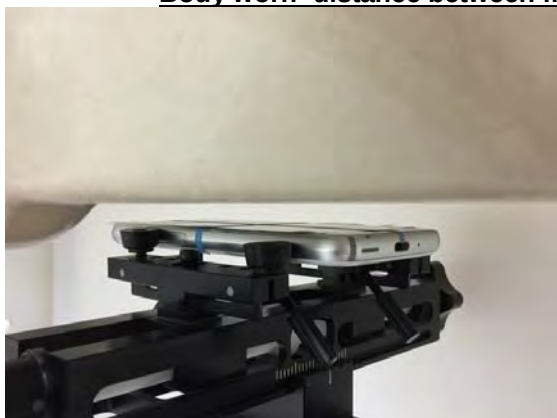
Fig.7 EUT Front side to flat phantom
