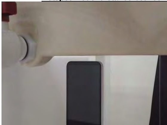
Fig.12 EUT Bottom side to flat phantom
