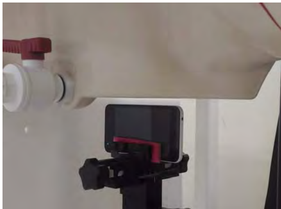
Fig.14 EUT Left side to flat phantom
