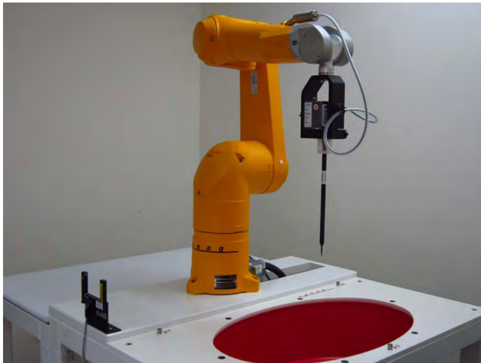
Fig.1 Photograph of the SAR measurement system
