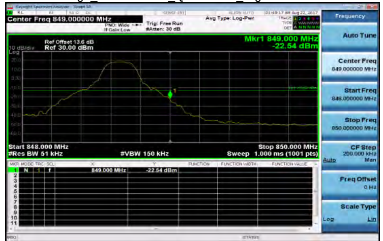
Band Edge Band5 5MHz QPSK 1 24 HighCH20625-846.5
