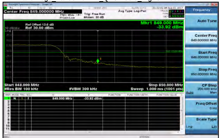
Band Edge Band5 10MHz QPSK 50 0 HighCH20600-844
