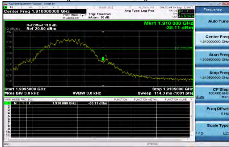
Band Edge GSM 1900MHz HighCH810-1909.8
