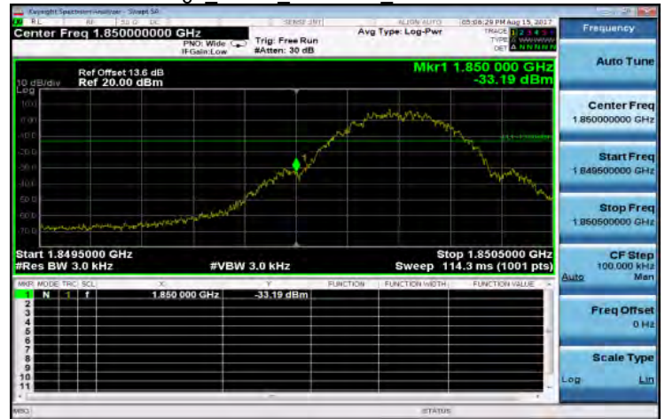
Band Edge GPRS 1900MHz LowCH512-1850.2
