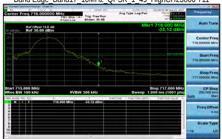
Band Edge Band17 10MHz QPSK 1 49 HighCH23800-711
