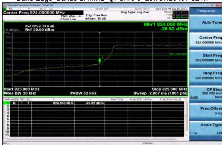
Band Edge Band5 1.4MHz QPSK 6 0 LowCH20407-824.7
