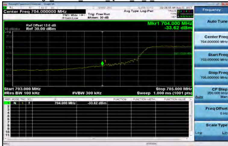
Band Edge Band17 10MHz QPSK 50 0 LowCH23780-709
