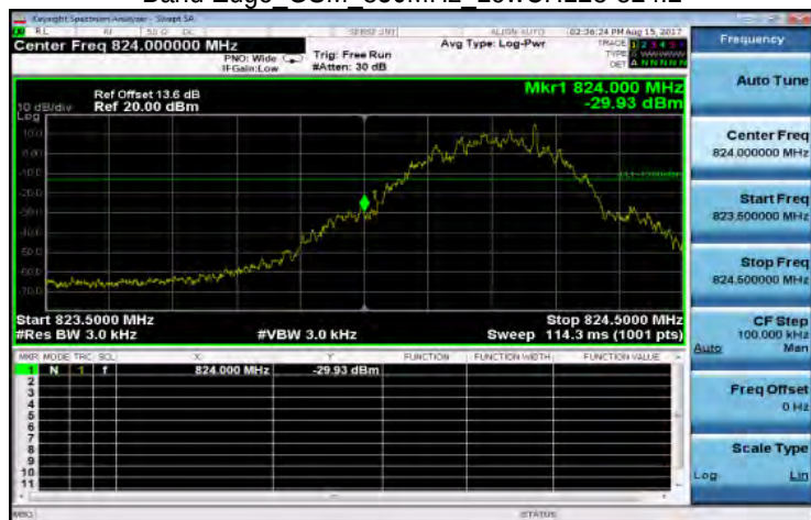
Band Edge GSM 850MHz LowCH128-824.2
