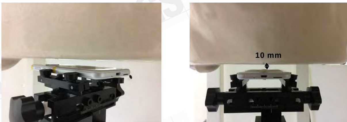
Fig.8 EUT Back side to flat phantom
