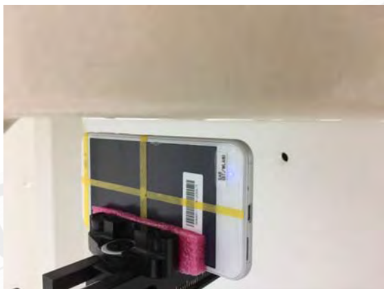
Fig.13 EUT Right side to flat phantom
