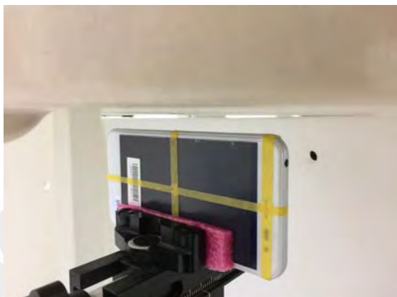
Fig.14 EUT Left side to flat phantom
