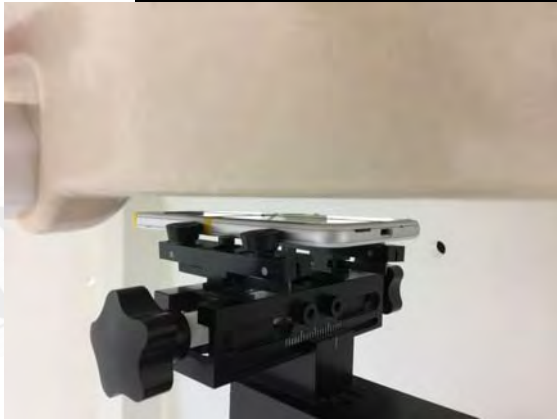
Fig.9 EUT Front side to flat phantom
