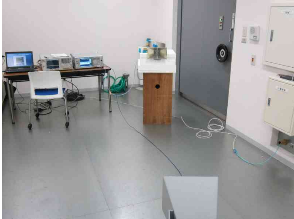
Test Setup for Generating the Radar Waveform
